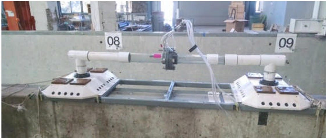
Figure 30. Standard caisson design for APEX tested at Hinsdale. This caisson design matches that tested in the ocean in 2014. Also seen in the image are the frame (grey, below the caissons), and the oscillating air column, and tygon tubing air lines used to measure air flow within the device (verify operation of the WEC)
