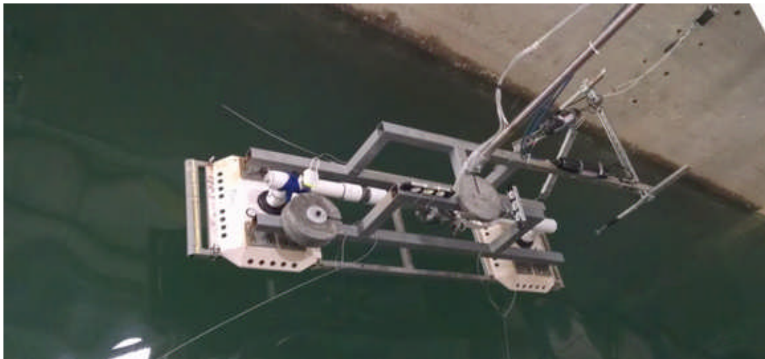
Figure 33. The “lift frame is shown, suspended via its vertical screw. Note, there are levels on the frame for viewing via underwater camera and ROV during testing and deployment. There are also two ADVs mounted aft of the WEC: one is in line with the WEC, and one is outboard, to starboard.
