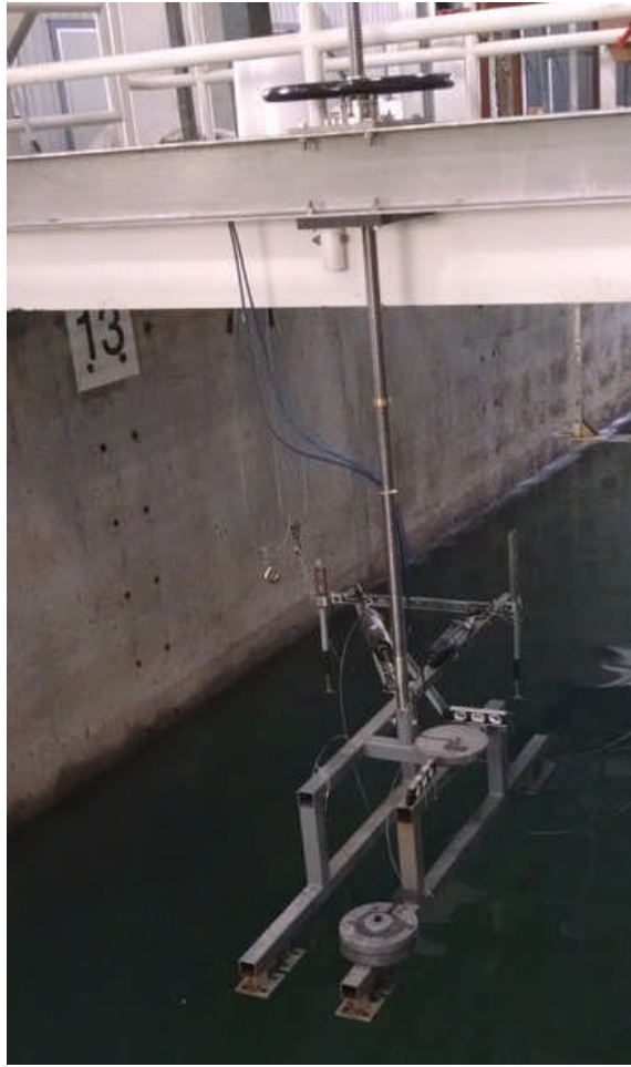
Figure 33. The “lift frame is shown, suspended via its vertical screw. Note, there are levels on the frame for viewing via underwater camera and ROV during testing and deployment. There are also two ADVs mounted aft of the WEC: one is in line with the WEC, and one is outboard, to starboard.
