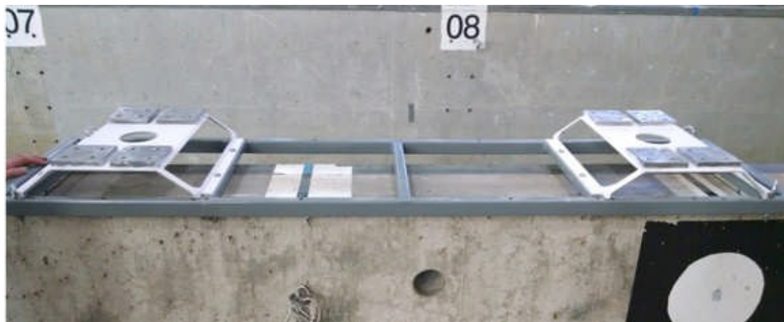
Figure 31. A stripped down version of the "skeleton" APEX device tested at Hinsdale. This WEC has the same frame as the standard WEC, but its caisson's have had most of the "sloped" surfaces removed, allowing water to flow through the caisson area / bag area more easily. Note, the air column is not present in this image.
