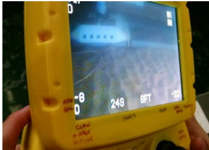
Figure 28. A typical live image from the ROV controller, showing ripples developed in the sediment after running waves. From this view, scour and accretion could be assessed relative to the horizontal, grey frame rails.
