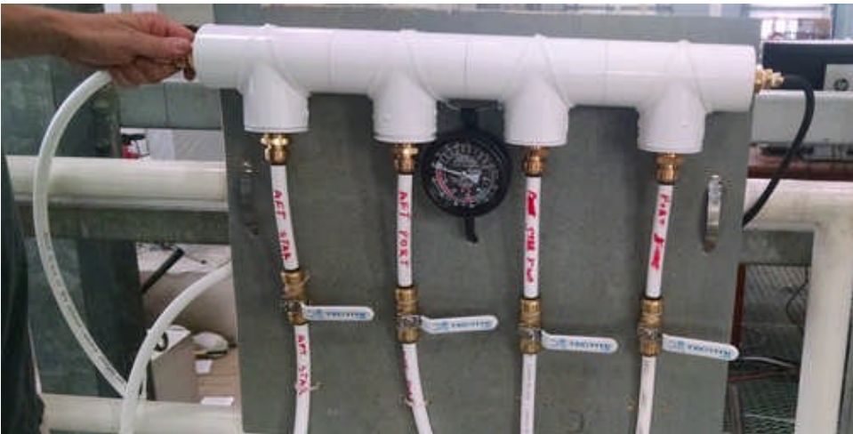
Figure 36. The vacuum manifold system used to measure and apply suction to each of the suction piles during deployment of the “suction pile” WEC.
