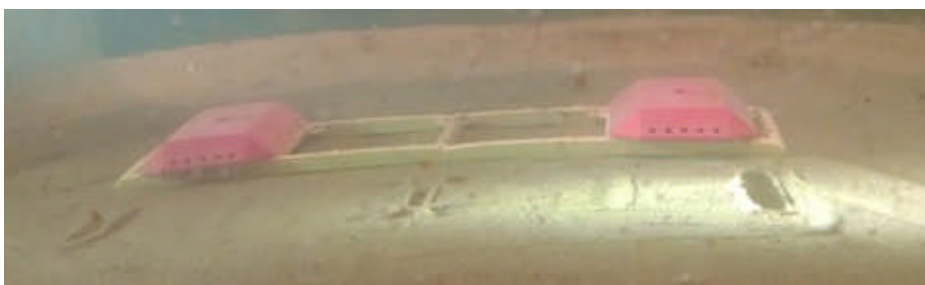
Figure 23. 1:25 standard APEX design on sand, behind scoured area. A scour trough can be seen at each end near the caisson to end rail gap. Sand build up at the central rail is also seen. This is after 15 minutes of wave A, Regime IV waves.
